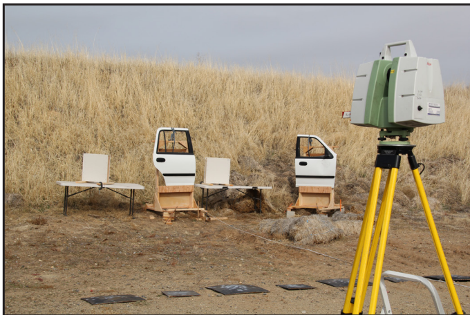
Leica Geosystems C10 ScanStation with Targets
